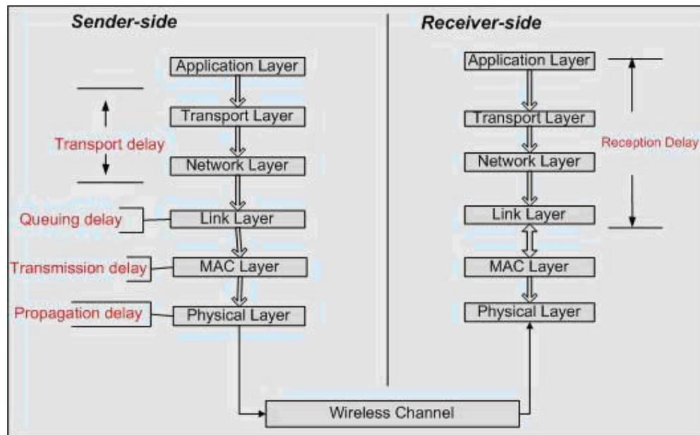
**Fig. 2.** Types of Packet Delay
